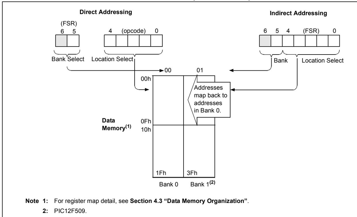
**FIGURE 4-8: DIRECT/INDIRECT ADDRESSING (PIC16F505)**
