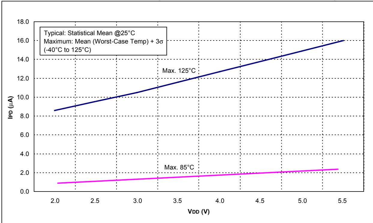
**FIGURE 11-5: TYPICAL WDT IPD vs. VDD**
