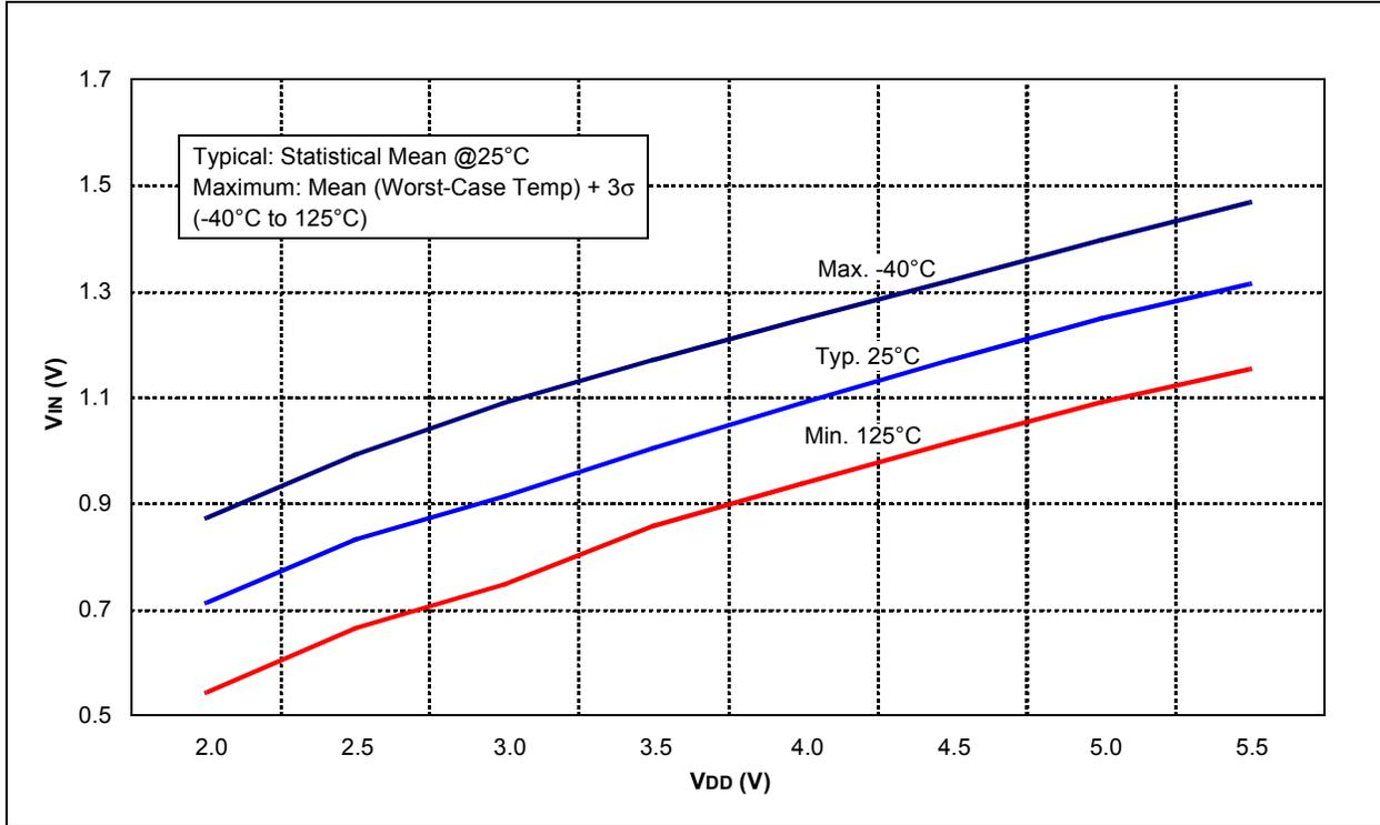
**FIGURE 11-13: SCHMITT TRIGGER INPUT THRESHOLD  $V_{IN}$  vs.  $V_{DD}$**
