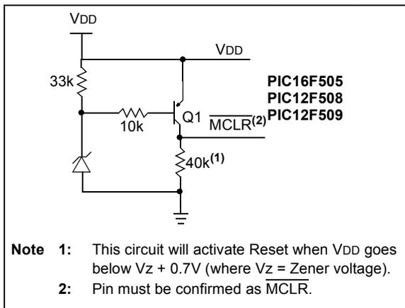
**FIGURE 7-13: BROWN-OUT PROTECTION CIRCUIT 2**
