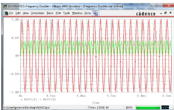
Figure 33. Frequency Doubler Response Graph Displayed in PSPICE
