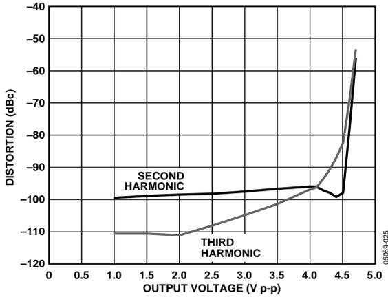
Figure 19. Distortion vs. Output Voltage @ 100 kHz,
