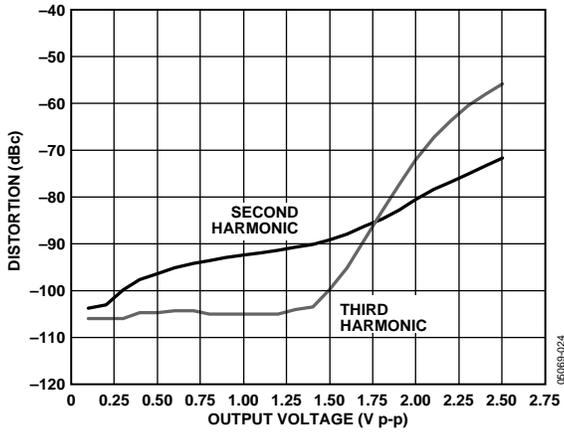
Figure 18. Distortion vs. Output Voltage @ 100 kHz,
