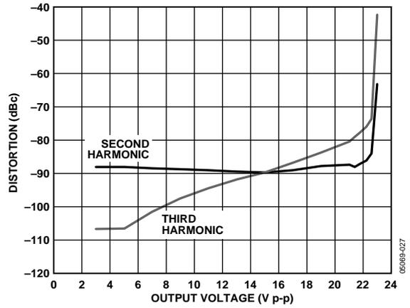
Figure 21. Distortion vs. Output Voltage @ 100 kHz,
