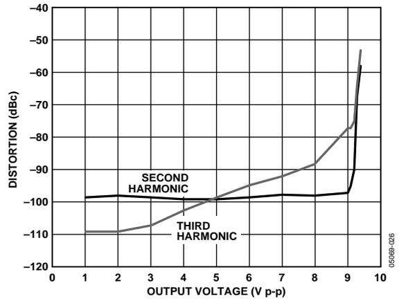
Figure 20. Distortion vs. Output Voltage @ 100 kHz,
