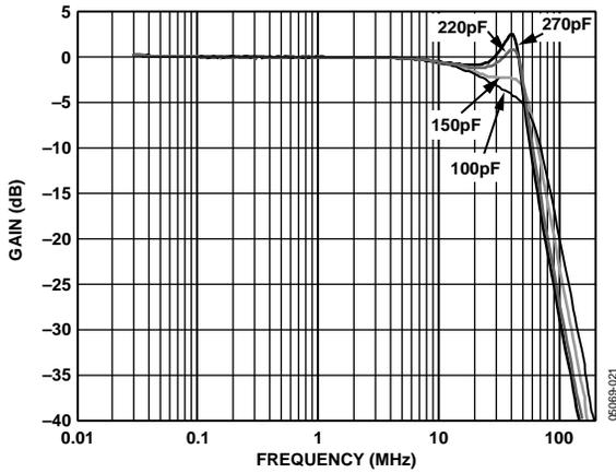
Figure 23. Capacitive Load Peaking Without Series Resistor
