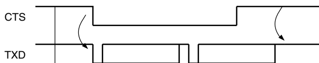
Figure 31-21. Transmitter Behavior when Operating with Hardware Handshaking
