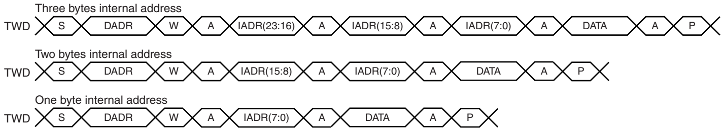
Figure 30-11. Master Write with One, Two or Three Bytes Internal Address and One Data Byte
