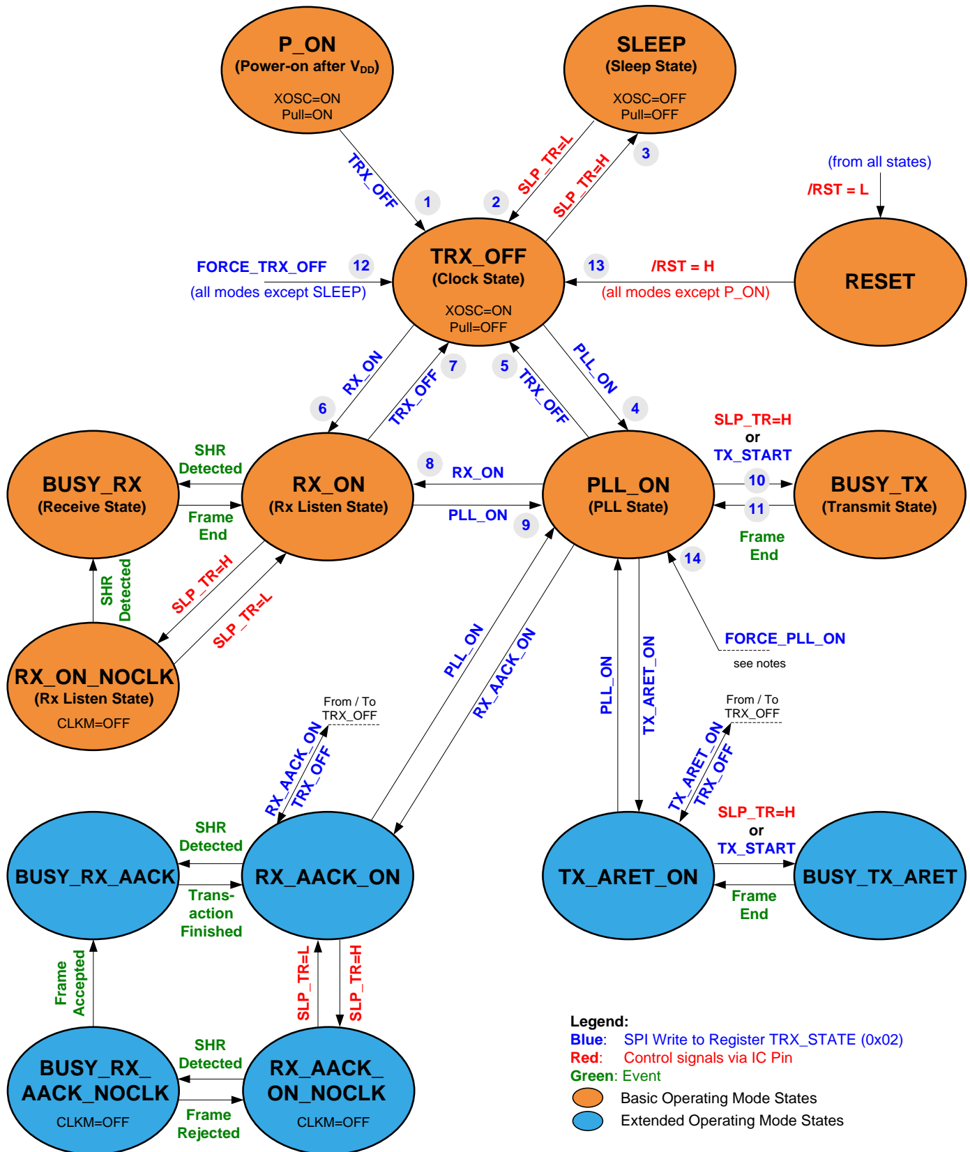
Figure 7-10. Extended Operating Mode State Diagram.
