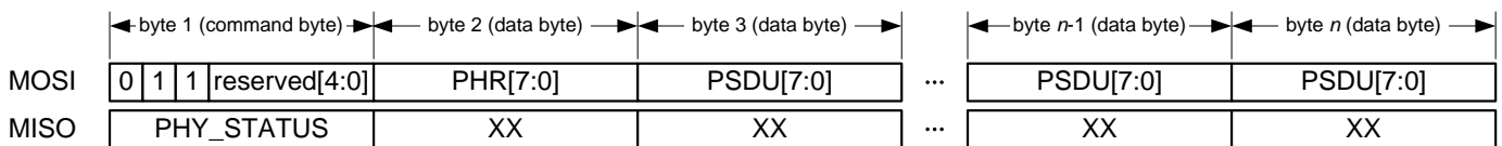
Figure 6-8. Packet Structure - Frame Write Access.
