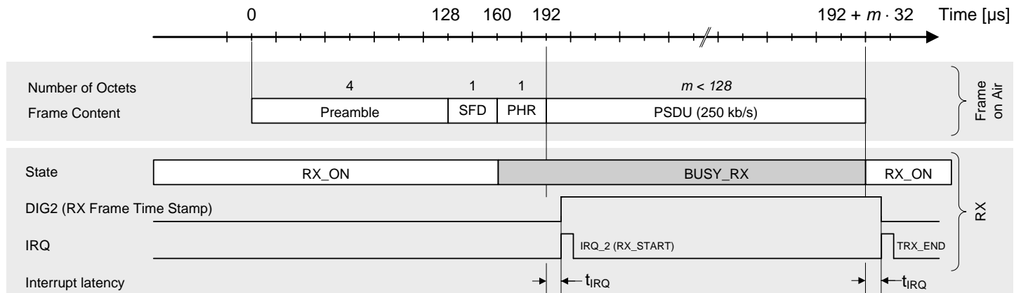
Figure 11-13. Timing of RX_START and DIG2 for RX Frame Time Stamping within 250kb/s O-QPSK mode.
