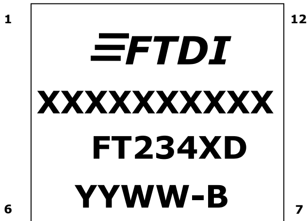
Figure 9.2 DFN-12 Package Markings
