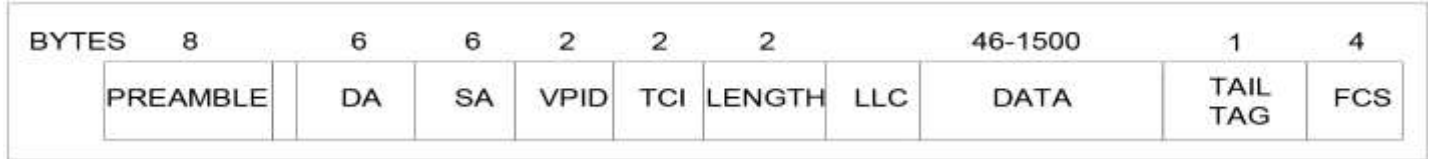
Figure 13. Tail Tag Frame Format
