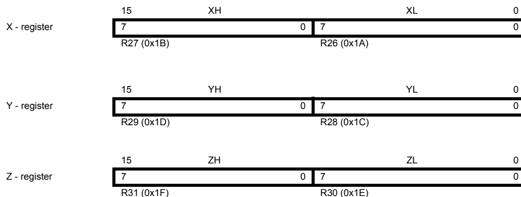
Figure 7-3. The X-, Y-, and Z-Registers
