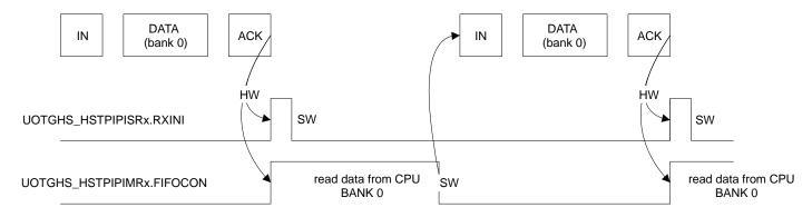
Figure 40-25. Example of an IN Pipe with 2 Data Banks
