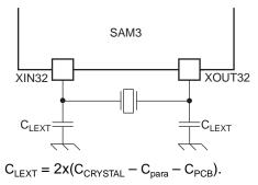
Where C<sub>PCB</sub> is the capacitance of the printed circuit board (PCB) track layout from the crystal to the SAM3 pin.
