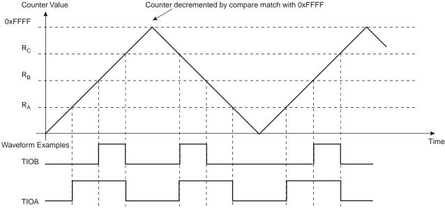
Figure 37-12. WAVSEL = 01 With Trigger
