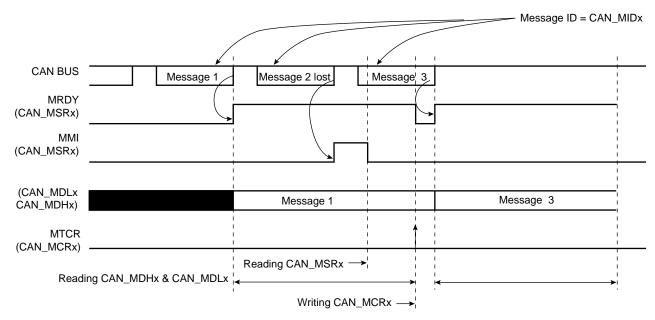
Note: In the case of ARM architecture, CAN\_MSRx, CAN\_MDLx, CAN\_MDHx can be read using an optimized ldm assembler instruction.
