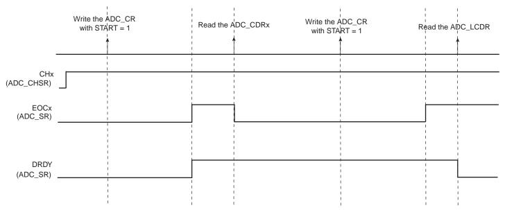
If the ADC\_CDR is not read before further incoming data is converted, the corresponding Overrun Error (OVREx) flag is set in the Overrun Status Register (ADC\_OVER).
