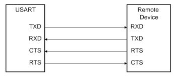
Setting the USART to operate with hardware handshaking is performed by writing the USART\_MODE field in the Mode Register (US\_MR) to the value 0x2.
