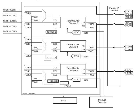
Note: The quadrature decoder logic connections are detailed in Figure 37-15 "Predefined Connection of the Quadrature Decoder with Timer Counters"
