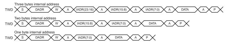
Figure 34-12. Master Read with One, Two or Three Bytes Internal Address and One Data Byte
