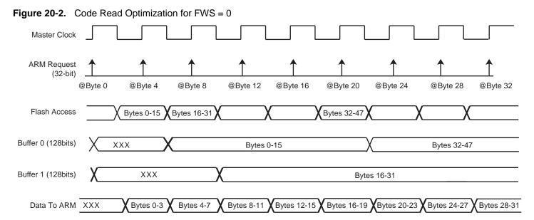
Note: When FWS is equal to 0, all the accesses are performed in a single-cycle access.
