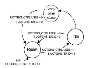
After a hardware reset, the UOTGHS device mode is in Reset state. In this state:
