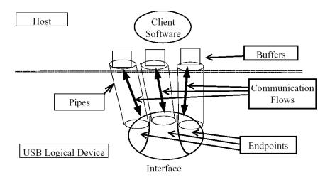
In host mode, the UOTGHS associates a pipe to a device endpoint, considering the device configuration descriptors.
