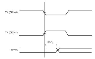
Figure 46-21. SSC Transmitter, TK as output and TF as input
