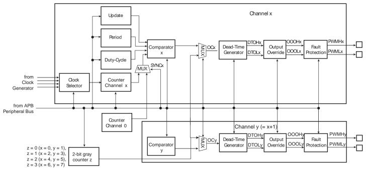
Each of the 8 channels is composed of six blocks:
