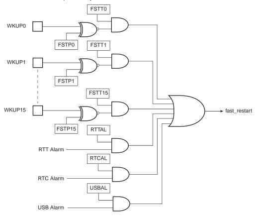
Each wake-up input pin and alarm can be enabled to generate a Fast Startup event by writing 1 to the corresponding bit in the Fast Startup Mode Register PMC\_FSMR.
