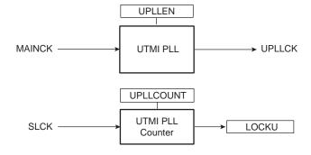
Whenever the UTMI PLL is enabled by writing UPLLEN in CKGR\_UCKR, the LOCKU bit in PMC\_SR is automatically cleared. The values written in the PLLCOUNT field in CKGR\_UCKR
