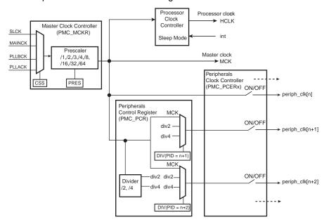
Figure 29-7. Peripheral Clock Divider Block Diagram
