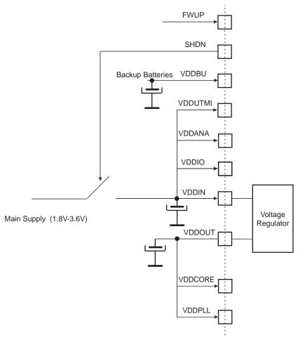
Note: Restrictions: With Main Supply < 3V, some peripherals such as USB and ADC might not be operational. Refer to the DC Characteristics of the product for actual possible ranges for such peripherals.
