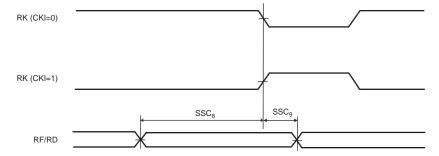
Figure 46-24. SSC Receiver, RK as input and RF as output
