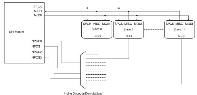
Figure 33-9. Chip Select Decoding Application Block Diagram: Single Master/Multiple Slave Implementation
