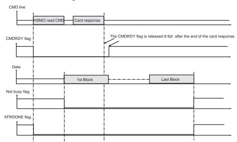
Figure 38-12. XFRDONE During a Read Access
