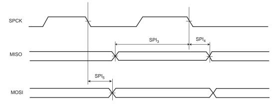
Figure 46-17. SPI Slave Mode with (CPOL=0 and NCPHA=1) or (CPOL=1 and NCPHA=0)
