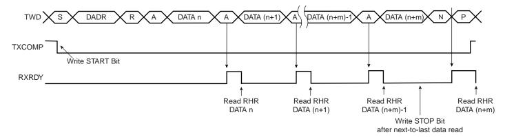
RXRDY is used as Receive Ready for the PDC receive channel.
