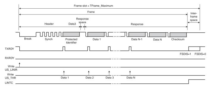
Figure 36-47. Master Node Configuration, NACT=SUBSCRIBE
