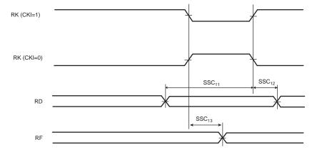
Figure 46-26. SSC Receiver, RK as output and RF as input
