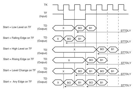
Figure 31-11. Receive Pulse/Edge Start Modes
