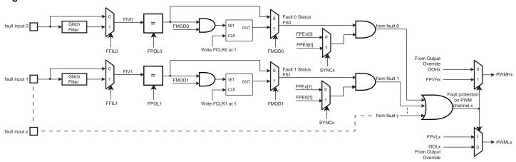
The polarity level of the fault inputs is configured by the FPOL field in the "PWM Fault Mode Register" (PWM\_FMR). For fault inputs coming from internal peripherals such as ADC, Timer Counter, to name but a few, the polarity level must be FPOL = 1. For fault inputs coming from external GPIO pins the polarity level depends on the user's implementation.
