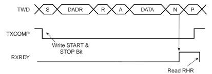
Figure 34-10. Master Read with Multiple Data Bytes
