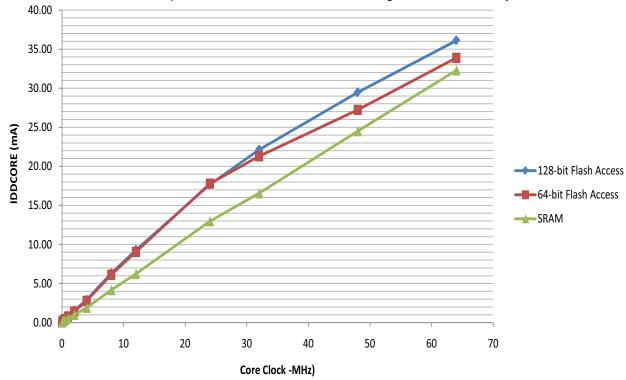
Table 46-12. Active Power Consumption with VDDCORE @ 1.62V running from Flash Memory or SRAM
