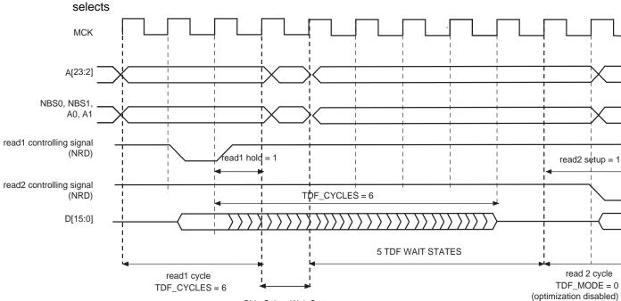
Figure 27-20. TDF Optimization Disabled (TDF Mode = 0). TDF wait states between 2 read accesses on different chip selects
