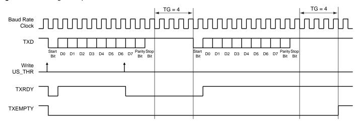
Table 36-10 indicates the maximum length of a timeguard period that the transmitter can handle in relation to the function of the Baud Rate.
