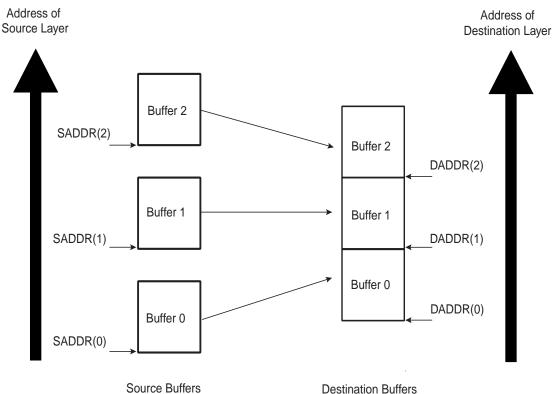
The DMAC transfer flow is shown in Figure 24-9 on page 367.
