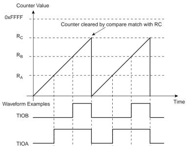
**Figure 37-9.** WAVSEL = 10 Without Trigger
