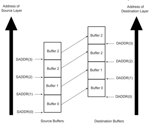
The DMAC transfer flow is shown in Figure 24-7 on page 363.
