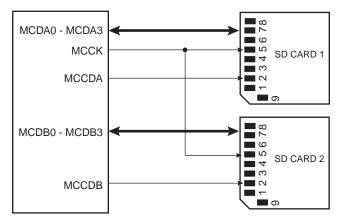
Note: When several HSMCI (x HSMCI) are embedded in a product, MCCK refers to HSMCIx\_CK,MCCDA to HSMCIx\_CDA, MCDAy to HSMCIx\_DAy, MCCDB to HSMCIx\_CDB, MCDBy to HSMCIx\_DBy.
