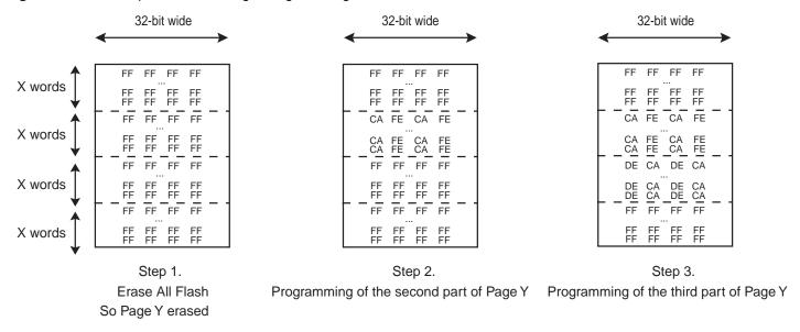
The Partial Programming mode works only with 128-bit (or higher) boundaries. It cannot be used with boundaries lower than 128 bits (8, 16 or 32-bit for example).
