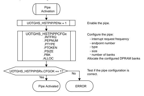
As long as the pipe is not correctly configured (UOTGHS\_HSTPIPISRx.CFGOK is zero), the controller cannot send packets to the device through this pipe.
