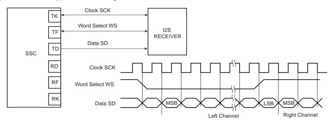
Figure 31-18. Codec Application Block Diagram
