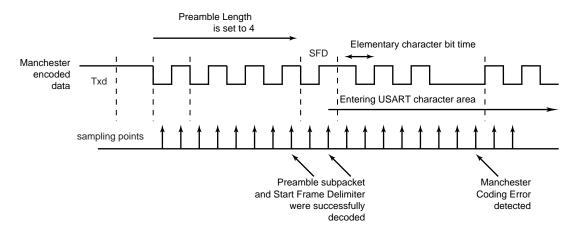
When the start frame delimiter is a sync pattern (ONEBIT field to 0), both command and data delimiter are supported. If a valid sync is detected, the received character is written as RXCHR field in the US\_RHR register and the RXSYNH is updated. RXCHR is set to 1 when the received character is a command, and it is set to 0 if the received character is a data. This mechanism alleviates and simplifies the direct memory access as the character contains its own sync field in the same register.
