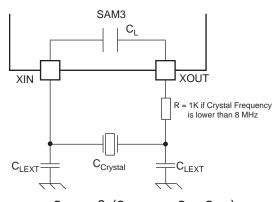
$C_{LEXT} = 2x(C_{CRYSTAL} - C_L - C_{PCB}).$
