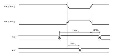
Figure 46-25. SSC Receiver, RK and RF as output
