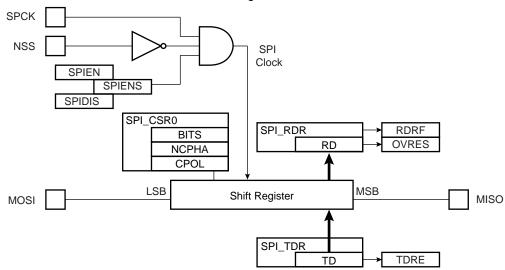
Figure 33-11. Slave Mode Functional Bloc Diagram
