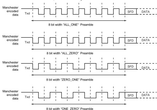
Figure 36-9. Preamble Patterns, Default Polarity Assumed
