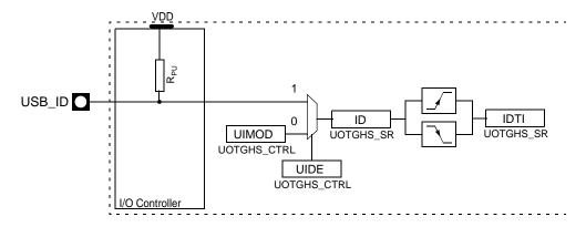
The USB mode (device or host) can be either detected from the UOTGID pin or software selected by writing to the UOTGHS\_CTRL.UIMOD bit, according to the UOTGHS\_CTRL.UIDE bit. This allows the UOTGID pin to be used as a general purpose I/O pin even when the USB interface is enabled.
