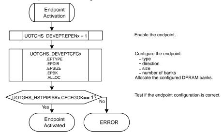
As long as the endpoint is not correctly configured (UOTGHS\_HSTPIPISRx.CFGOK is zero), the controller does not acknowledge the packets sent by the host to this endpoint.
