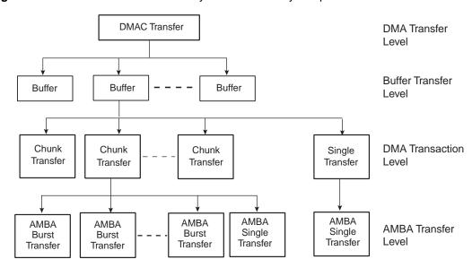
Figure 24-2. DMAC Transfer Hierarchy for Non-Memory Peripheral
