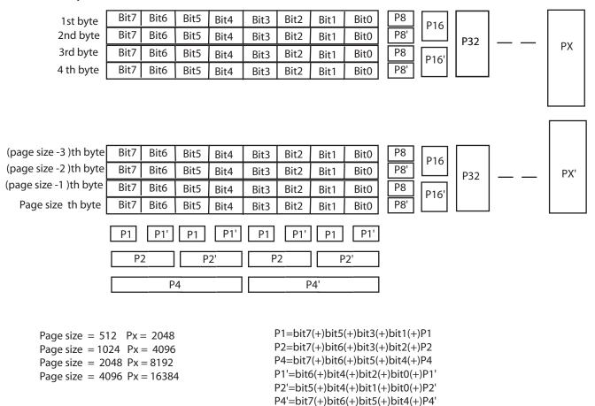
To calculate P8' to PX' and P8 to PX, apply the algorithm that follows.
