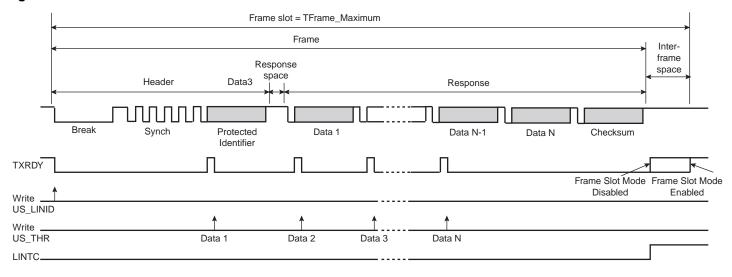
36.7.8.14 LIN Errors Bit Error This error is generated in Master of Slave node configuration, when the USART is transmitting and if the transmitted value on the Tx line is different from the value sampled on the Rx line. If a bit error is detected, the transmission is aborted at the next byte border.
