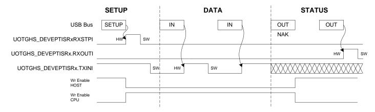
A NAK handshake is always generated on the first status stage command.
