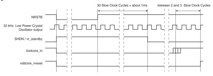
Note: periph\_nreset, ice\_reset and proc\_nreset are not shown, but are asserted low thanks to the vddcore\_nreset signal controlling the Reset controller.
