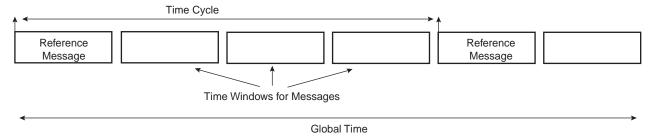
Time Trigger Mode is enabled by setting the TTM field in the CAN\_MR register. In Time Triggered Mode, as in Timestamp Mode, the CAN\_TIMESTP field captures the values of the internal counter, but the MTIMESTAMP fields in the CAN\_MSRx registers are not active and are read at 0.
