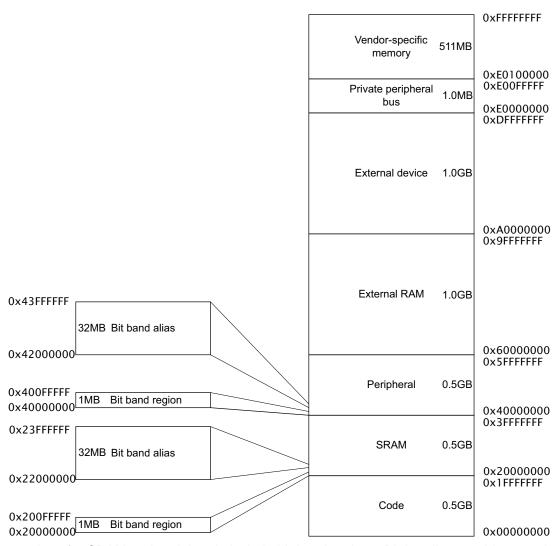
The regions for SRAM and peripherals include bit-band regions. Bit-banding provides atomic operations to bit data, see "Bit-banding" on page 75.
