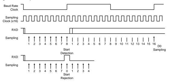
Figure 36-13. Asynchronous Character Reception
