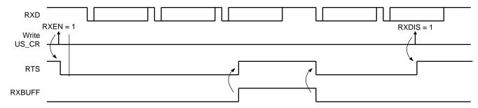
Figure 36-29 shows how the transmitter operates if hardware handshaking is enabled. The CTS pin disables the transmitter. If a character is being processing, the transmitter is disabled only after the completion of the current character and transmission of the next character happens as soon as the pin CTS falls.
