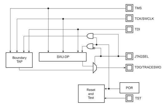
Figure 13-1. Debug and Test Block Diagram
