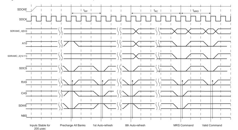
Figure 26-1. SDRAM Device Initialization Sequence
