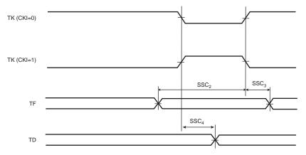
Figure 46-22. SSC Transmitter, TK and TF as input
