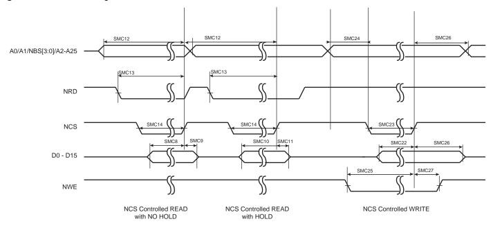
Figure 46-29. SMC Timings - NRD Controlled Read and NWE Controlled Write
