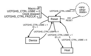
After a hardware reset, the UOTGHS is in the Reset state. In this state:
