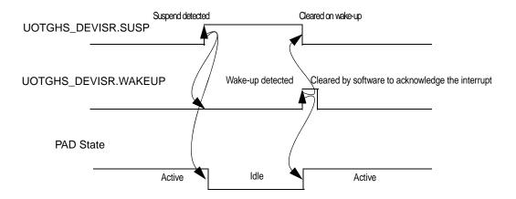
The UOTGHS\_DEVISR.SUSP bit is set and the Wake-Up Interrupt (UOTGHS\_DEVISR.WAKEUP) bit is cleared when a USB "Suspend" state has been detected on the USB bus. This event automatically puts the USB pad in Idle state. The detection of a non-idle event sets UOTGHS\_DEVISR.WAKEUP, clears UOTGHS\_DEVISR.SUSP and wakes up the USB pad.
