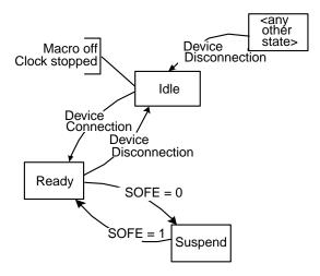
After a hardware reset, the UOTGHS host mode is in the Reset state.
