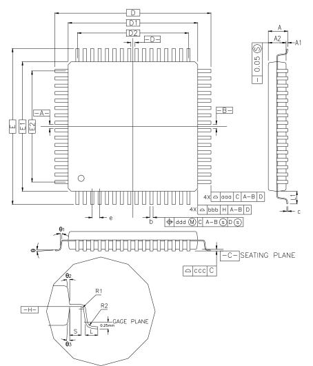
COTROL DIMENSIONS ARE IN MILLIMETERS.
