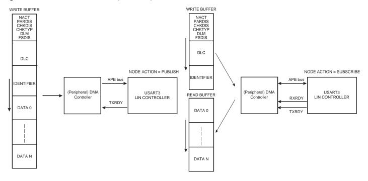
Figure 36-53. Master Node with PDC (PDCM = 0)
