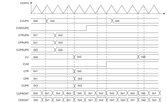
Figure 39-15. Comparison Waveform
