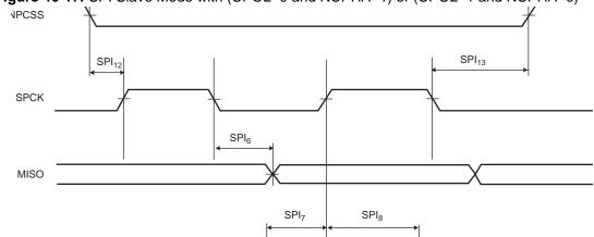
Figure 46-18. SPI Slave Mode with (CPOL = NCPHA = 0) or (CPOL= NCPHA= 1)
