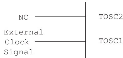
Figure 14-15. Timer/Counter2 External Clock Connections
