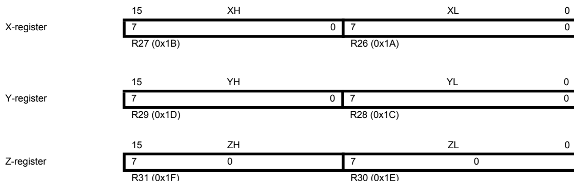
Figure 6-3. The X-, Y-, and Z-registers
