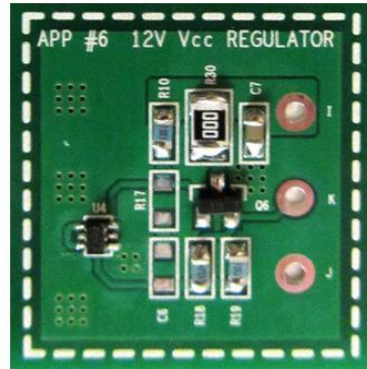
Built as 12 volt Regulator
