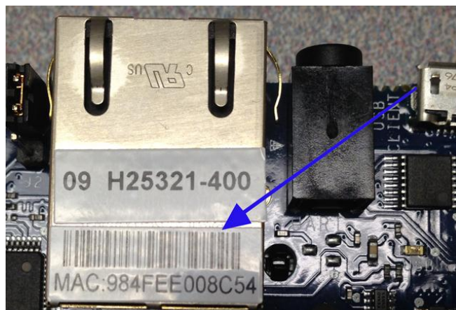
Figure 28. Location of MAC Address on Target System Ethernet Port
