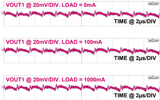
FIGURE 23. PWM1 OUTPUT RIPPLE, MODE = 5V (CCM)
