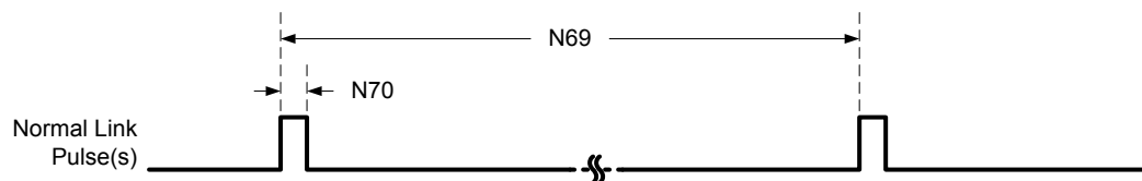
Figure 27-38. 10Base-TX Normal Link Pulse Timing
